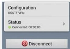
“Connected” in the **Status** area along with a timer increasing in value indicates a successful connection.
